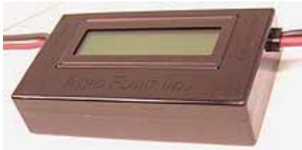
will handle voltage to 60V, amperage to 100 A, wattage up to 5,000W, and NiCad Amp-hour Capacity up to 9 Ah . This is my most important piece of equipment. It is the only way to know for sure what kind of power your system is really generating.
