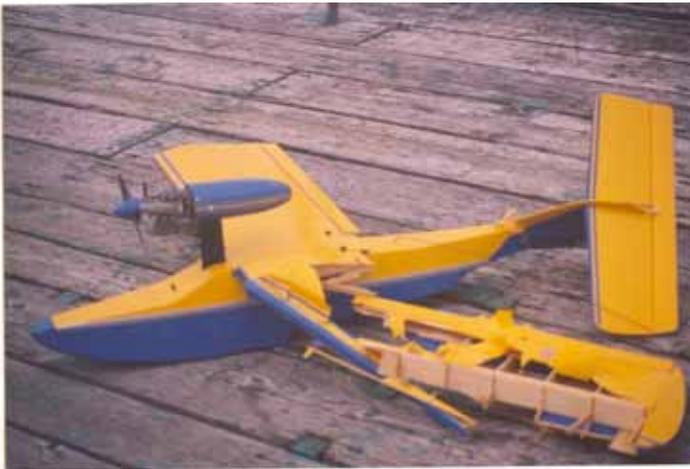
Bill worked at rebuilding the wing during the winter (which took many weeks). He found someone to laser cut a set of ribs and used a cardboard rocket tube as a replacement leading edge for the damaged panel to match the opposite wing.
